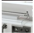
The hinged, transparent front safety guard is electronically controlled.
